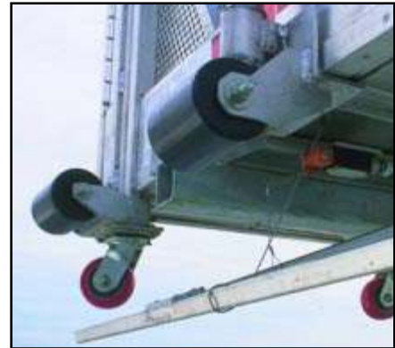
Photo above shows non-marking building face rollers. Many permanent platforms require extendable building face rollers (See photo at top of page P-4).
