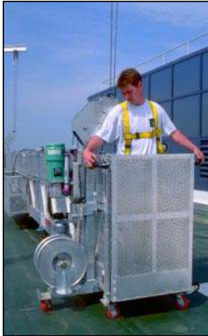
Highrise maintenance worker is demonstrating how the adjustable end of the platform will extend past the stirrup to reach that extra three feet (1 m) of glass.
