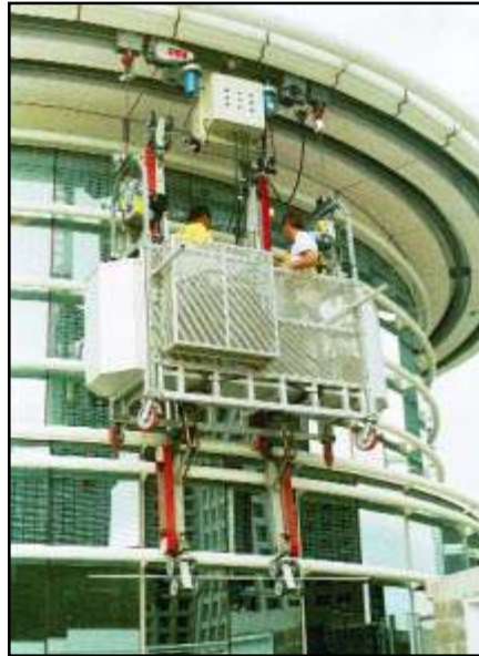
In order for the various Pro-Bel permanent powered suspended platforms to by-pass the accent pipe sections on the Garage Rotunda, Podium Rotunda, and Tower, special custom hydraulic retractable "ski rollers" that unfold to a vertical mode in front of the platform facilitate vertical travel up and down the face of the Enron building. These pipes would otherwise be difficult to circumvent with a conventional style platform.
