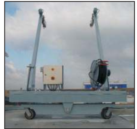
Pro-Bel Model PT 3008 powered trackless trolley supported on hard rubber tired wheels travels freestanding fully balanced on concrete bearing surface (or similar) cast on top of the roof finish (360° slewing and luffing capability).
