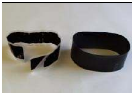
Collar flashing components: mastic sealant tape and heavy wall rubber tubing with its own integral adhesive liner.
