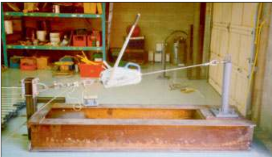
The static load test in the above photo, which applies force using a heavy duty cable come-along, was conducted to show that Pro-Bel wall and roof anchors comply with standards that require the anchors be capable of resisting without fracture and/or pull-out a force of 5000 lbs (22.2 kN). A similar test is performed on-site to verify strength of epoxy adhesive roof anchors.
