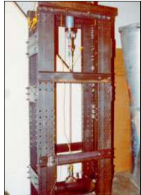
Photo shows 8'-0" (2440 mm) high apparatus used for shock (drop) testing of Pro-Bel safety U-Bar anchors. A 220 lb. (100 kg) weight was connected to the anchor using a steel test lanyard and dropped a distance of 4'-0" (1220 mm). A series of anchors employing different securements were tested and peak forces up to 18,522 lbs (8400 kg) were generated without fracture to any part of the anchors.
